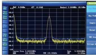
Display the spectrums when change the RBW settings with different color trace
